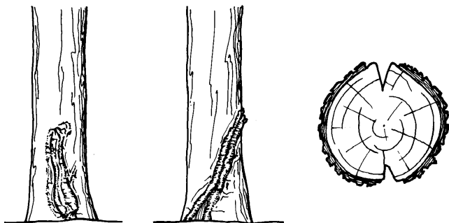
FIGURE 4.7. Appearance of frost crack on standing tree and in cross-section.
