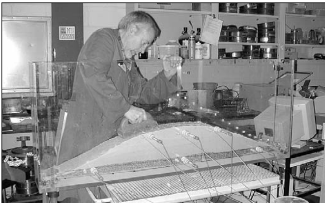
Construction of a 2-dimensional model dam.
