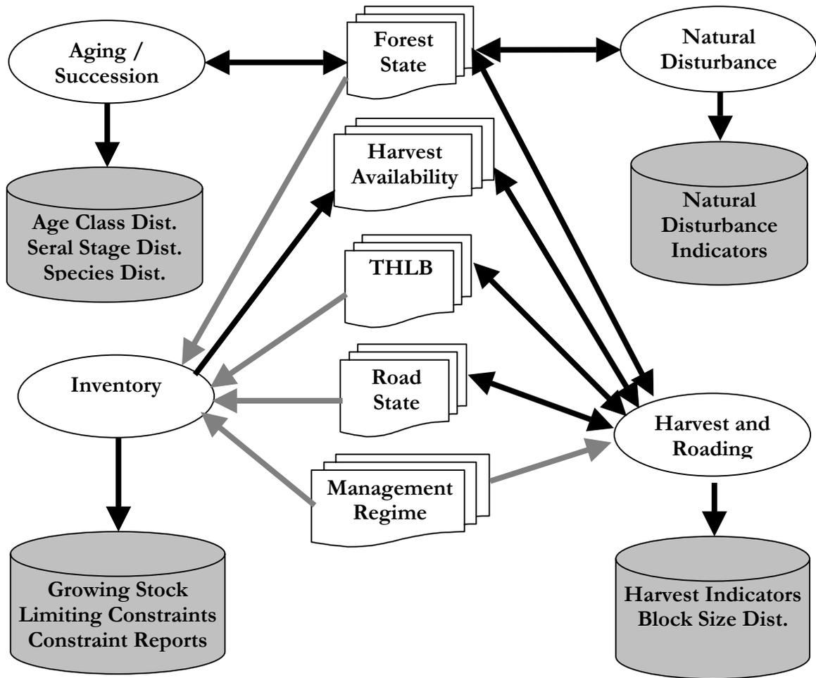
Figure 3. Overall conceptual design of the Morice Landscape Model landscape dynamics. Each main modeled process is shown as an oval, while the main parts of the landscape state (represented as spatial data layers and tables) are shown in the centre, and output files are shown as grey drums. Arrows indicate whether a process depends on and/or modifies the connected landscape state, or produces output.
