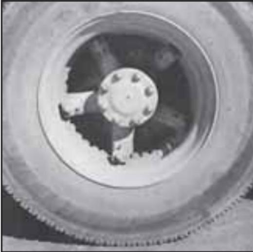
*Demountable rim mounted on cast spoke wheel*
