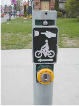
Bike activated traffic signals and other amenities encourage people to ride more frequently
