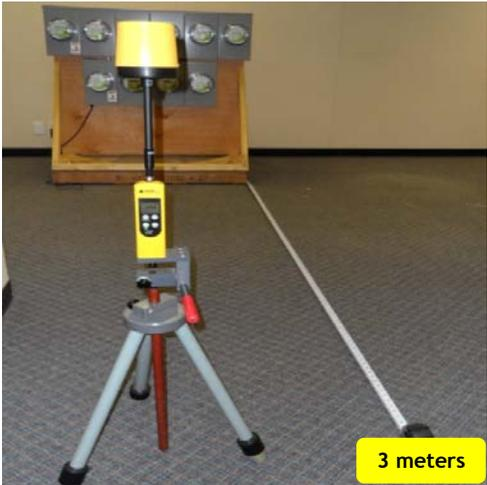
Probe at 3 meters from the smart meter bank
