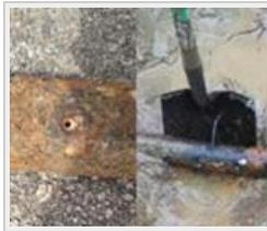
In Nakusp, a 1/8" puncture in a water main was located in March 2012. It is estimated that repairing this hole in a 2" galvanized steel line at a pressure of approximately 40 psi will result in a savings of nearly 5,000,000 litres annually.
