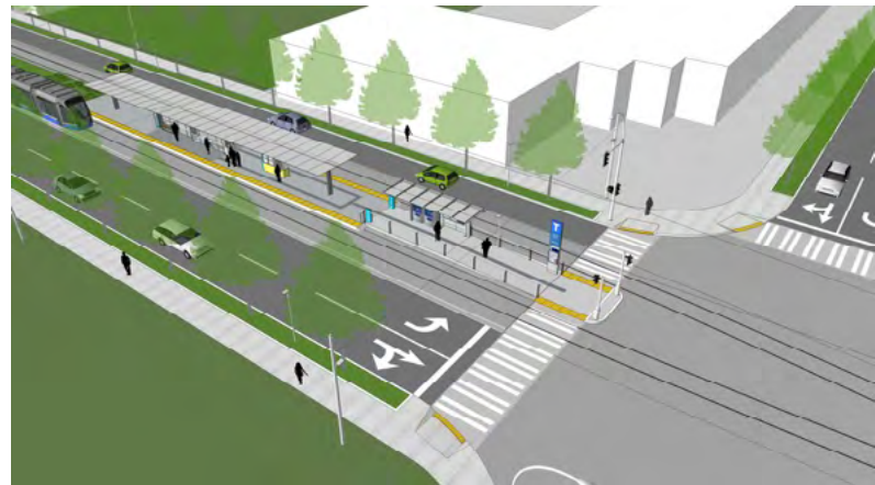
Figure 4 Sample Centre Platform LRT Stop
