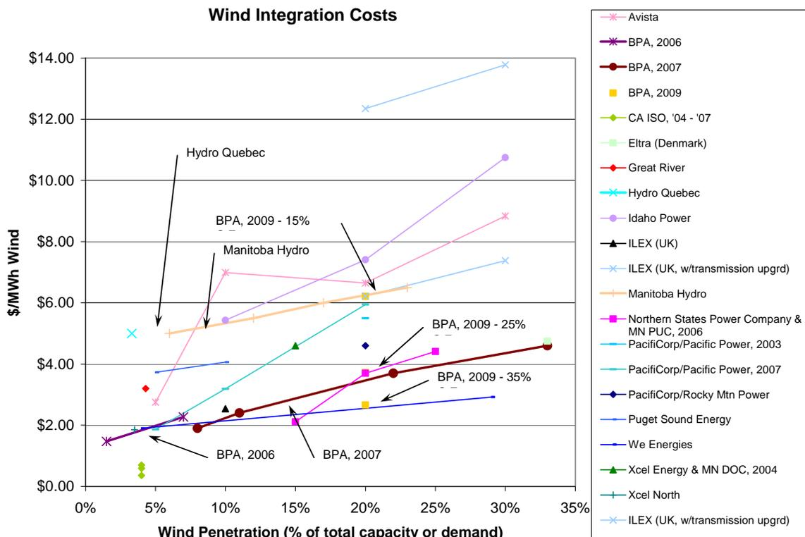
Of the utilities shown in Figure F3-4, it is of interest to further examine the wind integration cost estimates of three utilities which have similar generation profiles to that of BC Hydro. These include Manitoba Hydro (**MH**), Bonneville Power Administration (**BPA**), and Hydro Quebec (**HQ**). Table F3-5 shows the peak load/capacity and generation mixes of these three utilities, and whether they are market-based or cost-based utilities.
