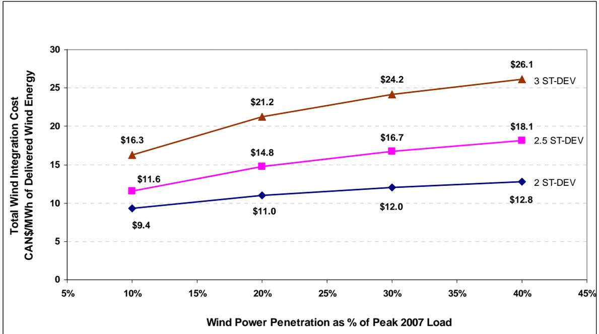
Figure F3-3 Variation of total wind integration cost with penetration and balancing reserve requirement levels for Case III aggregation scenario (25% Peace Region, 25% North Coast, 25% S&E Interior, and 25% Vancouver Island).
