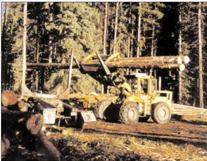
*A front-end loader is used to load logs onto a logging truck.*
